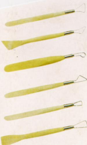
The large triangular tool defines wide inclined areas. Shape and position features with the flat round end.
